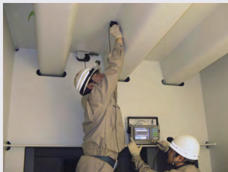
Steel plate floor automatic ultrasonic testing equipment (SAUT) A nondestructive inspection technique to detect fatigue cracks occurring inside steel plates
