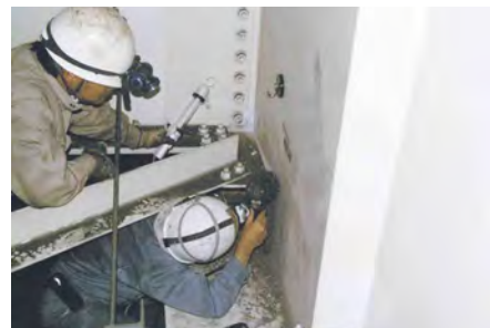
Magnetic particle flaw detection tests on steel floor plates
