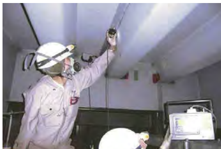
Ultrasonic flaw detection tests on steel floor plates
