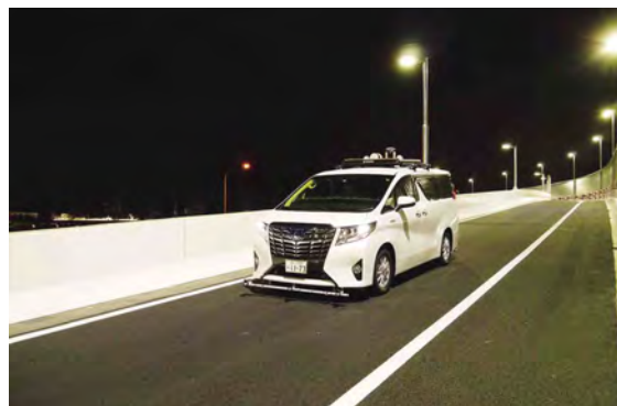
Measurement conducted by illuminance measuring vehicle
