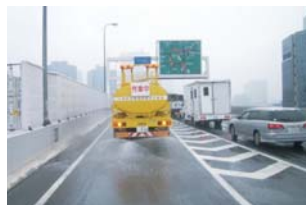
Scattering deicing agent (salt water) on the road surface
