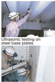
Magnetic particle examination conducted on steel girders
