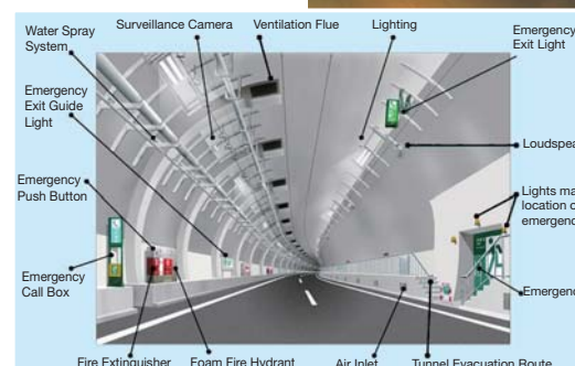
Yamate Tunnel disaster prevention equipment
